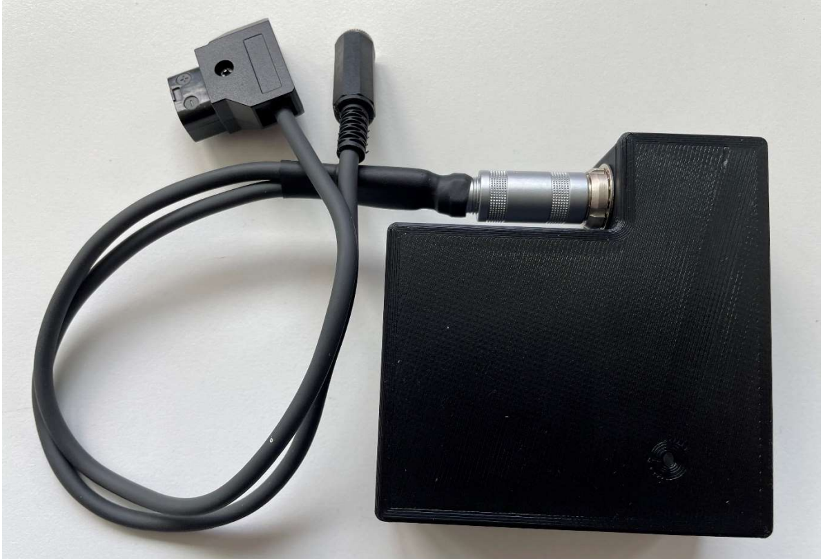
Figure 12 MACK Sony camera sender control system module with case
