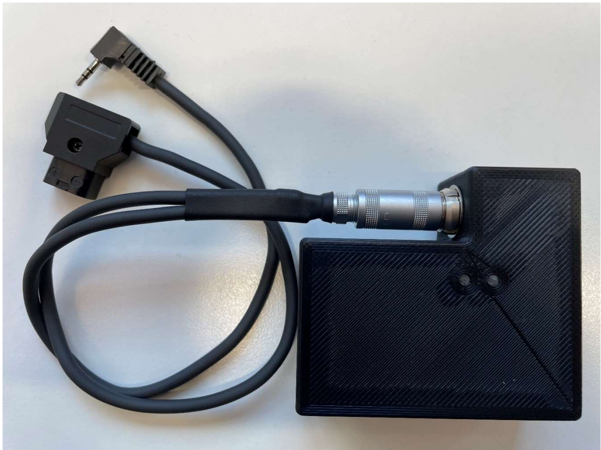
Figure 13 Realistic MACK Sony camera receiver control system module with case
